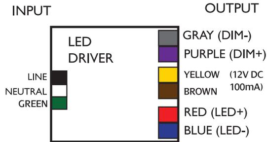
Both output positive and negative connectors are equivalent (same electrical point)
