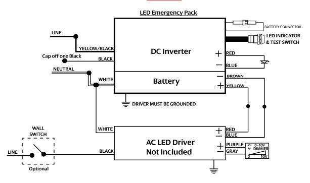
Input Voltage: 120-347V, 50.60Hz • Surge Rating 3Kv
