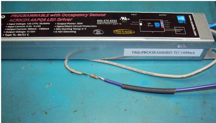
After soldering the resistor in place, the heat-shrink-tubing should be moved over the resistor and its solder joints, and hot air applied to cause the tubing to shrink. The end result is shown in Figure 3 below. As you can see, the tubing covers all solder joints, and is positioned with the resistor somewhat in the middle of the tubing.
