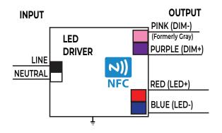
Note: Gray (-) dimming wire has been changed to pink per the 2020 NEC section 410.69 and NEMA.
