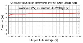
Emergency LED Driver comes in a single metal enclosure with a separate miniature illuminated test switch status indicator. This Linear Emergency LED Driver is suitable for installation in sealed and gasketed fixtures. The maximum remote mounting distance to the LEDs is 18 feet. The Linear Emergency LED Driver metal case should be grounded. Stranded copper wires, 18 AWG 600 V, 105 °C are required for installation. The unit will self-activate when AC power is applied for the first time.
