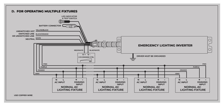
A.) The wiring diagrams shown depict full functionality utilizing the 0 - 10 V Auto Dimming feature.
