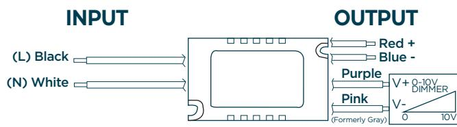
**Note:** Gray (-) dimming wire has been changed to pink per the 2020 NEC section 410.69 and NEMA.
