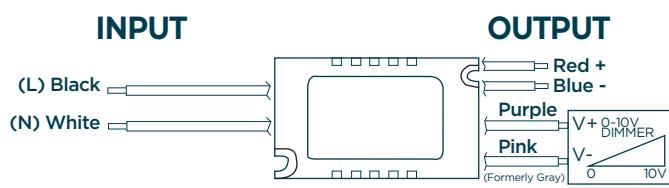
**Note:** Gray (-) dimming wire has been changed to pink per the 2020 NEC section 410.69 and NEMA.
