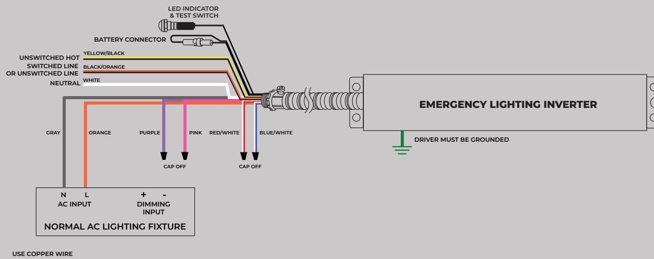
**C. IF THE 0 - 10 V AUTO DIMMING FEATURE IS USED, BUT EXTERNAL 0 - 10 V DIMMING CTRL IS NOT USED, THEN ONLY CAP OFF THE RED/WHITE AND BLUE/WHITE WIRES.**
