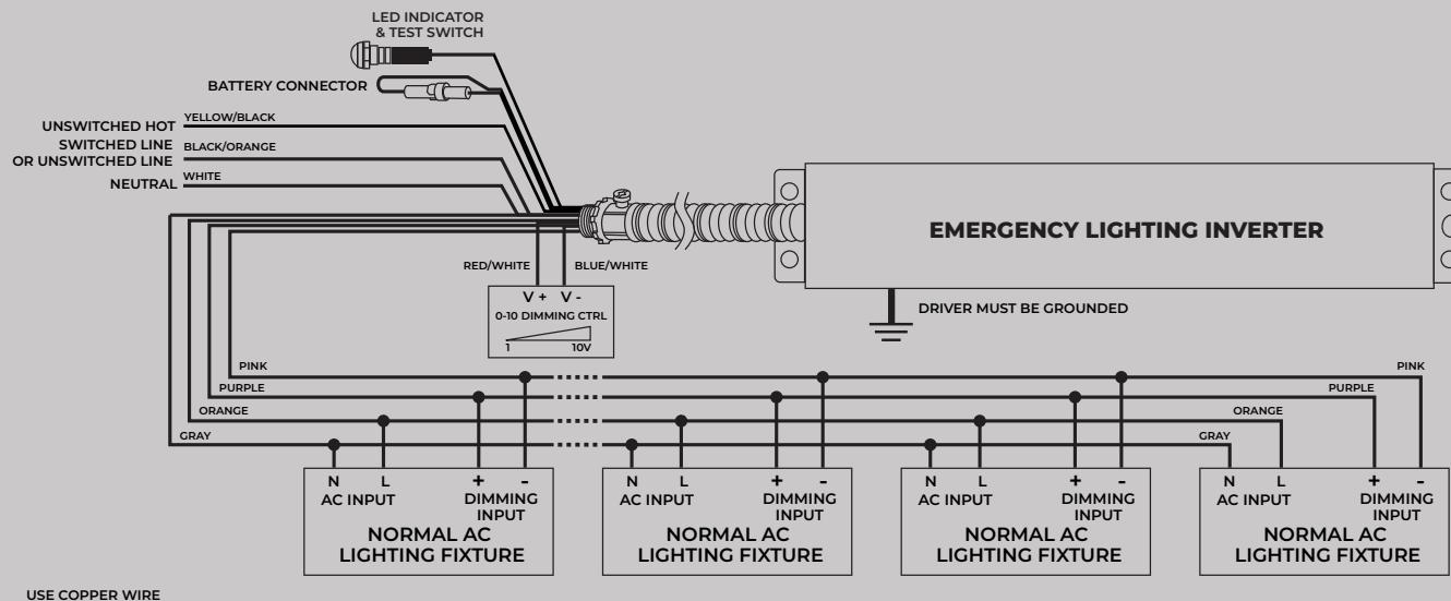
**A.)** The wiring diagrams shown depict full functionality utilizing the 0 - 10 V Auto Dimming feature.
